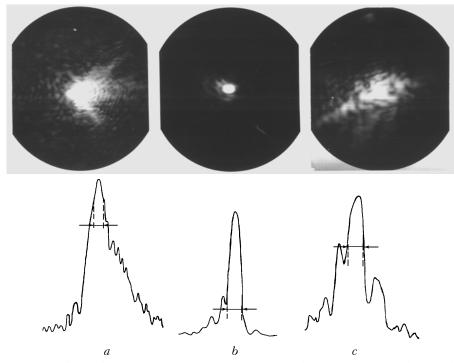
FIG. 4. The photographs of the focal spots and the densitograms of the radiation, reflected from the nonlinear medium and passed again through the optical channel. The diameter of the extended beam is equal to 150 mm, (a) and 75 mm, (b, c). The wave front on the last photographs was distorted additively by the heating of the area of the optical channel.
