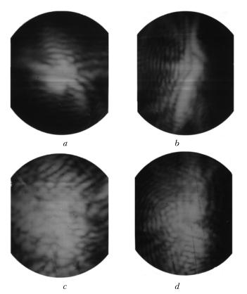
FIG. 3. The photographs of the focal spots of the beam radiation with  $\emptyset = 75 \text{ mm}$ , (a, b) and 150 mm, (c, d) with the thermal heating of the separate area of the optical channel, (b) at the 4 m shortened transportation channel, (c) and the 24 m complete one, (d). The photographs are in about the same scale relative to the diffraction angle.
