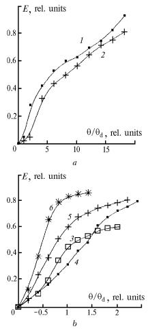
FIG. 2. The angular distribution of the radiation energy, incident on the nonlinear medium (curves 1, 2), (a); the output control laser beam (curve 3), reflected and passed again through the optical channel (curves 4–6), (b); the diameter of the beam is equal to 150 mm (curves 2, 4) and 75 mm (curves 1, 5, and 6); the curve 5 was obtained at heating separate areas of the optical channel.
