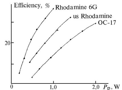
FIG. 2. Conversion efficiency of dye lasers versus pumping power in 6G (R6G), unsubstituted Rhodamine (UR), ocsathyn-17 (OC-17) dye solutions in non-selective optical cavity.
