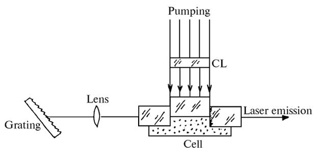
FIG. 3. Optical arrangement of a dye laser.
