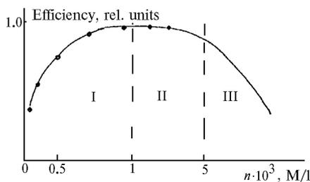
FIG. 1. Conversion efficiency of dye laser versus active medium concentration (Rhodamine 6G in ethanol).
