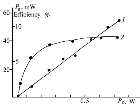
FIG. 4. Output power (1) and conversion efficiency (2) of a dye laser as a function of pumping power.
