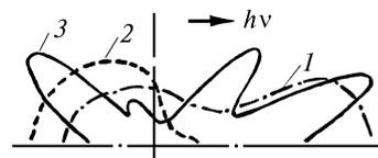
FIG. 1. Typical scattering phase functions: dumbbell-shaped (curve 1); pear-shaped (curve 2); and camomile-shaped scattering phase function (curve 3).
