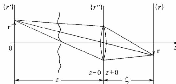
FIG. 1. Model of the image transfer through the turbulent atmosphere:  $r'$  is the point source coordinate in the object plane  $\{r'\}$ ;  $r''$  is the coordinate in the lens plane;  $r$  is the coordinate in the image plane;  $z$  is the distance between the object plane  $\{r'\}$  and a lens;  $\zeta$  is the distance between the image plane  $\{r\}$  and a lens;  $\zeta \approx f$  at  $f \ll z$ , where  $f$  is the focal length of a lens.
