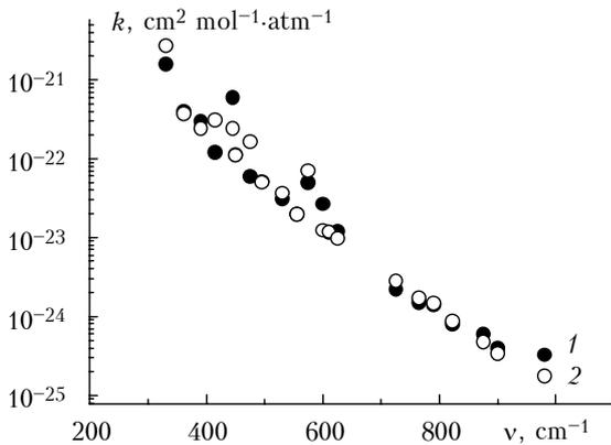
FIG. 4. The values of the absorption coefficient in the gas mixture  $\text{H}_2\text{O}-\text{N}_2$  at  $T = 296$  K; experimental (Ref. 20) (1) and calculated in accordance with the theory of line wings (Refs. 14 and 15) (2).
