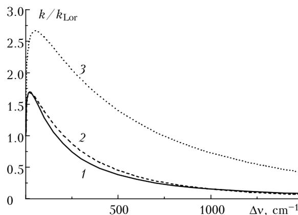
FIG. 1. Deviations from the Lorentz line shape for the Thomas-Nordstrom empirical line shapes  $P_{\text{H}_2\text{O}} = 0.02 \text{ atm}$ ,  $P_{\text{H}_2\text{O}+\text{N}_2} = 1 \text{ atm}$ ;  $\nu_0 = 199.935 \text{ cm}^{-1}$  (1),  $\nu_0 = 1600.849 \text{ cm}^{-1}$  (2),  $\nu_0 = 3499.883 \text{ cm}^{-1}$  (3).
