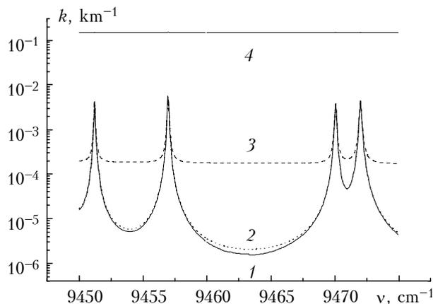
FIG. 2. Absorption coefficient of the gas mixture  $\text{H}_2\text{O}-\text{N}_2$  for several values of the Lorentz line shape widths at  $T = 296\text{ K}$ ,  $\rho_{\text{H}_2\text{O}} = 16.5\text{ g/m}^3$ :  $\Delta\nu = 20\text{ cm}^{-1}$  (1),  $\Delta\nu = 100\text{ cm}^{-1}$  (2),  $\Delta\nu = 1000\text{ cm}^{-1}$  (3), and  $\Delta\nu = 10000\text{ cm}^{-1}$  (4).
