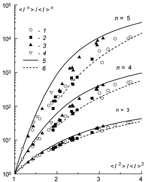
Fig. 4. Normalized moments of the intensity of 3rd, 4th, and 5th orders:  $\Delta = 26$  mm (1); 36 mm (2); 120 mm (3); 208 mm (4); moments of the lognormal distribution (5); moments of the K-distribution (6).
