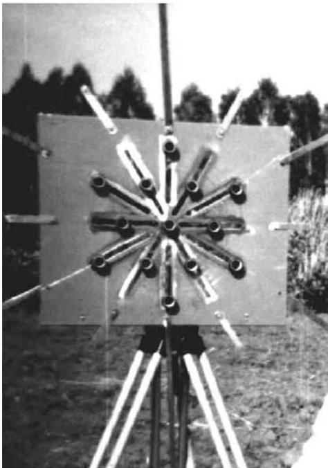
Fig. 1. The array of the corner-cube reflectors.
