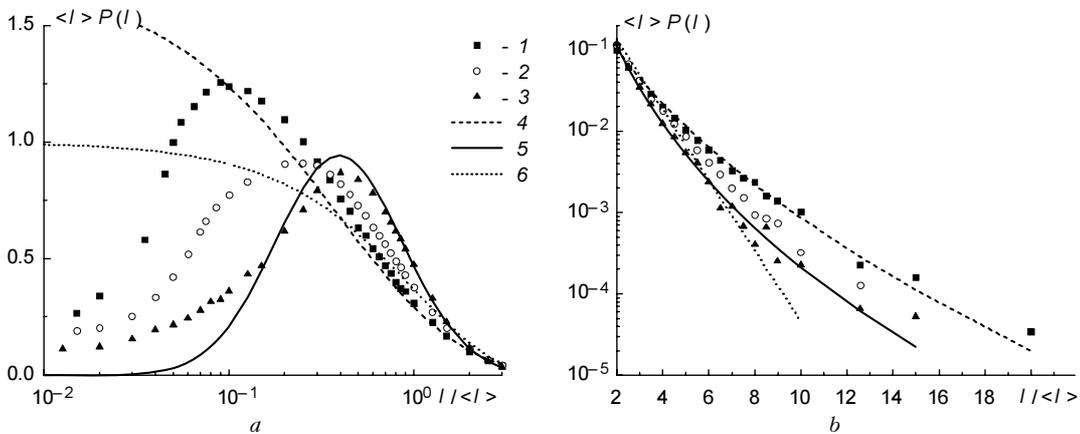
Fig. 3. Histograms of the normalized intensity values for  $\beta_0(L) = 7$ .  $\Delta = 26$  mm (1); 36 mm (2); 120 mm (3); K-distribution corresponding to the histogram 1 (4); lognormal distribution corresponding to the histogram 3 (5); exponential distribution (6).
