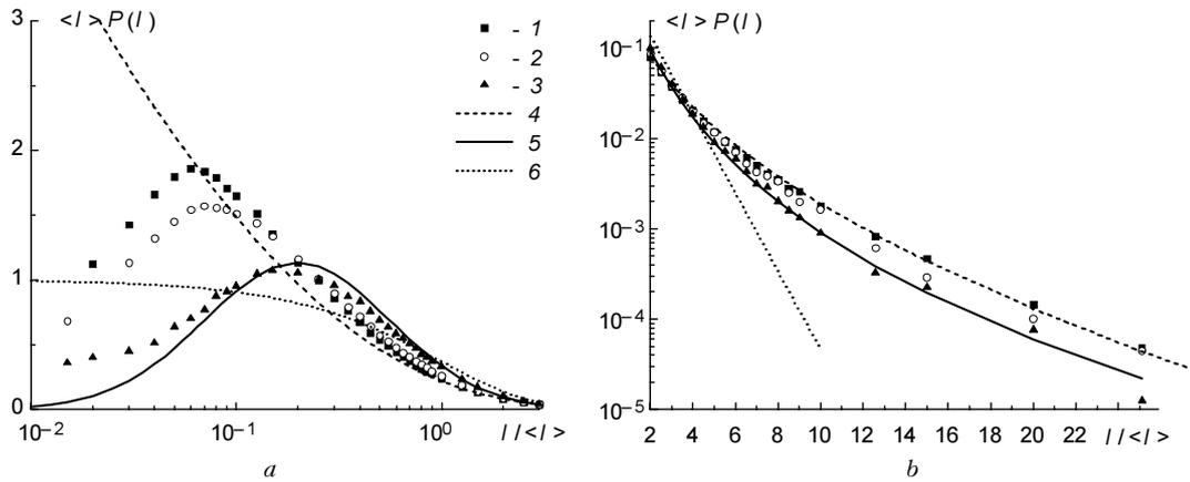
Fig. 2. Histograms of the normalized intensity values for  $\beta_0(L) = 1$ .  $\Delta = 26$  mm (1); 36 mm (2); 208 mm (3); K-distribution corresponding to the histogram 1 (4); lognormal distribution corresponding to the histogram 3 (5); exponential distribution (6).
