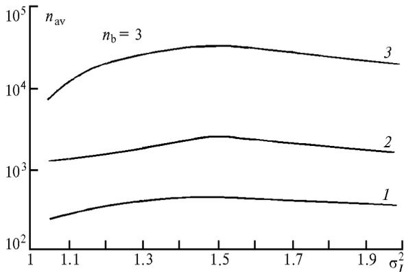
Fig. 2. The dependence of  $n_{av}$  on  $\sigma_I^2$  for  $K$ -distribution of optical wave intensity fluctuations:  $P_{sk} = 10^{-3}$  (curve 1);  $P_{sk} = 10^{-4}$  (curve 2);  $P_{sk} = 10^{-6}$  (curve 3).
