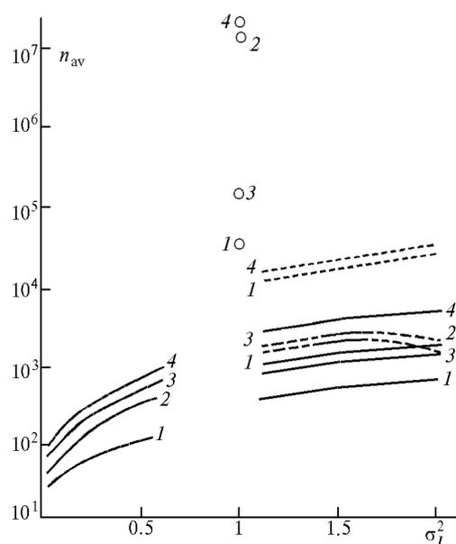
**Fig. 1.** Dependence of  $n_{av}$  on  $\sigma_I^2$ : lognormal distribution (solid curves),  $K$ -distribution (dashed curves); exponential distribution (circles);  $n_b = 1, \dots, P_{sk} = 10^{-4}, \dots, n_{thr} = 6$  (curve 1);  $n_b = 1, \dots, P_{sk} = 10^{-6}, \dots, n_{thr} = 9$  (curve 2);  $n_b = 10, \dots, P_{sk} = 10^{-4}, \dots, n_{thr} = 24$  (curve 3);  $n_b = 10, \dots, P_{sk} = 10^{-6}, \dots, n_{thr} = 28$  (curve 4).
