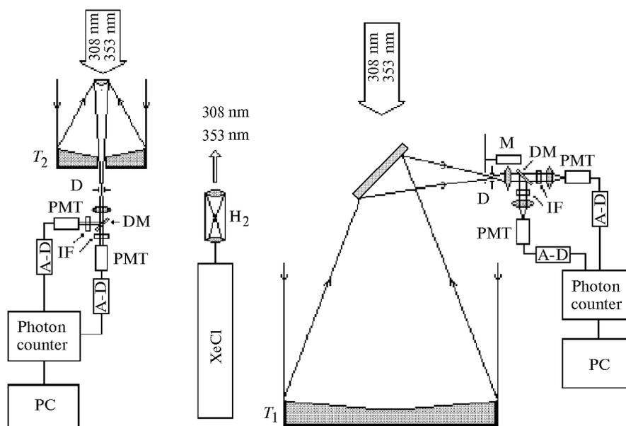
**Fig. 1.** Block diagram of the modified UV lidar: XeCl excimer laser ( $\lambda = 308$  nm); H<sub>2</sub> SRS cell ( $m_2$ ); large and small receiving telescopes ( $T_1$  and  $T_2$ ); field stop diaphragm (D); mechanical chopper (M); FEU-130 photomultiplier tube (PMT); interference filter (IF); dichroic mirror (DM); amplifier-discriminator (A-D); personal computer (pC).
