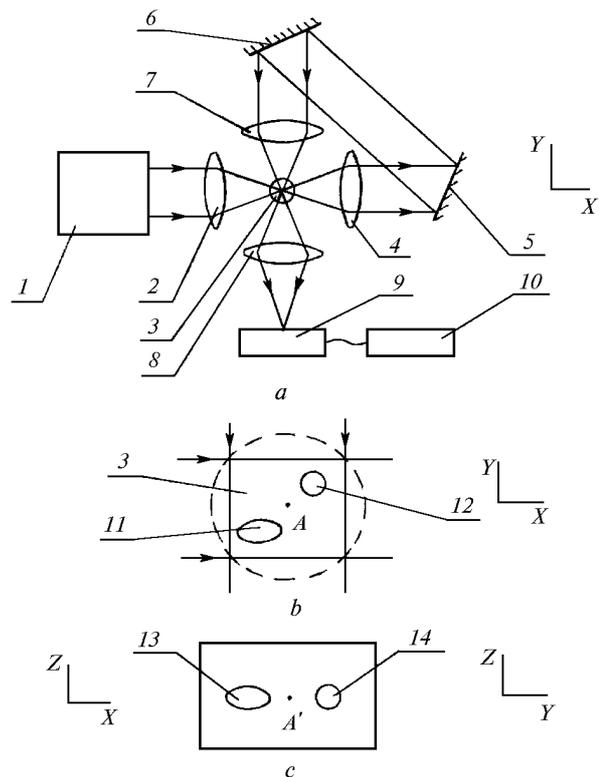
**Fig. 1.** Formation of projections of a particle onto two mutually perpendicular planes: overall diagram (a), view of the beam intersection region (b), view of the recording plane (c): illuminator 1; objectives 2, 4, 7, 8; particle flux 3; mirrors 5, 6; video camera 9; processing block 10; particle 11; first and second images of the particle 12, 13; image of the first image 14.
