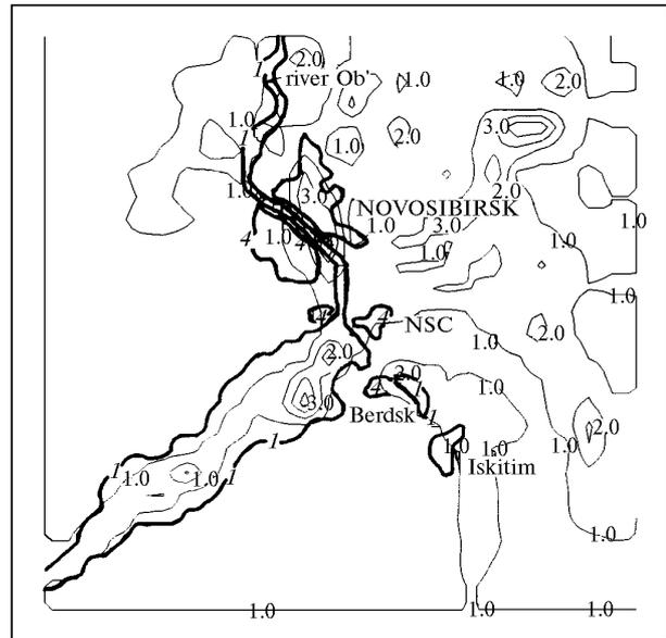
Fig. 2. The field of pollutant concentration (50 m above the level of relief) in the region at the southwest background flux (10 m/s). Fall, 6:00 LT.
