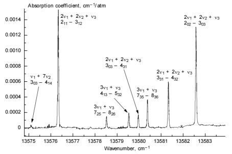
Fig. 2. Water vapor absorption spectrum in the 13575-13583 cm<sup>-1</sup> region.
