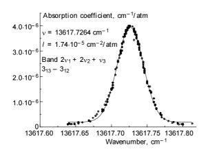
Fig. 3. Spectral dependence of the absorption coefficient for the  $13617.7264 \text{ cm}^{-1}$  line: measured values (circles), the result of Voigt profile fitting (solid curve).
