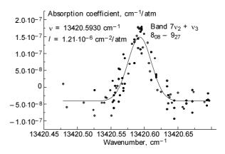
**Fig. 4.** Spectral dependence of the absorption coefficient for the  $13420.5930 \text{ cm}^{-1}$  line corresponding to the transition to the (071) highly excited bending state: measured values (circles), the result of Voigt profile fitting (solid curve).
