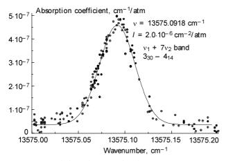
**Fig. 5.** Spectral dependence of the absorption coefficient for the  $13575.0918 \text{ cm}^{-1}$  line corresponding to the transition to the (170) highly excited bending state: measured values (circles), the result of Voigt profile fitting (solid curve).
