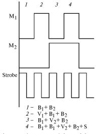
Fig. 2. The diagram of operation of the modulators and strobe to obtain a signal.
