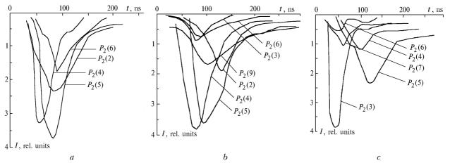
**Fig. 5.** Time behavior of intensity of separate lines of the  $P_2$  transition in the mixture SF<sub>6</sub>:H<sub>2</sub> = 7:1 at different pressure: 0.82 (*a*), 0.344 (*b*), and 0.096 atm (*c*).
