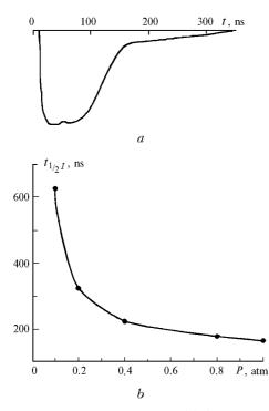
**Fig. 4.** Oscillogram of radiation pulse (*a*) (p = 0.344 atm) and pressure dependence of the pulse duration at halfmaximum (*b*) in the mixture SF<sub>6</sub>:H<sub>2</sub> = 7:1.
