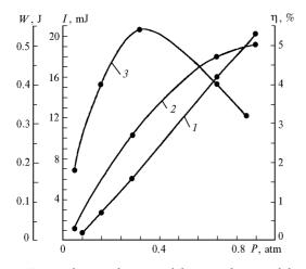
**Fig. 1.** Energy dissipated in a gas (1), emitted energy (2), and efficiency (3) as functions of the active medium pressure  $SF_6:H_2 = 7:1$ .
