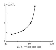
**Fig. 2.** Output laser energy as a function of E/p.  $I_{\rm b}$  and  $I_{\rm d}$  are the radiation energy in the case of active medium excitation by *e*-beam and by an *e*-beam-initiated discharge, respectively. Mixture SF<sub>6</sub>:H<sub>2</sub> = 7:1, p = 0.184 atm.
