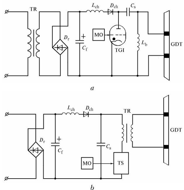
**Fig. 1.** The pump circuits with thyatron switch (a) and with a transistor switch (b): transformer TR, rectifier  $D_r$ , filtering capacitor  $C_f$ , by-pass inductance  $L_b$ , charging inductance  $L_{ch}$  (choke), charging diode  $D_{ch}$ , energy storage capacitor  $C_s$ , thyatron TGI, master oscillator MO, gas-discharge tube GDT, and a transistor switch TS.
