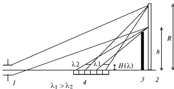
Fig. 1. Optical arrangement of the focal monochromator based on a holographic lens.
