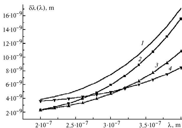
Fig. 3. Spectral resolution at different optical parameters:  $d = 1$  (1, 3, 4) and 0.5 mm (2);  $R = 3$  (1, 2, 3) and 2 cm (4);  $h = 1$  (1, 2, 4) and 2 cm (3).
