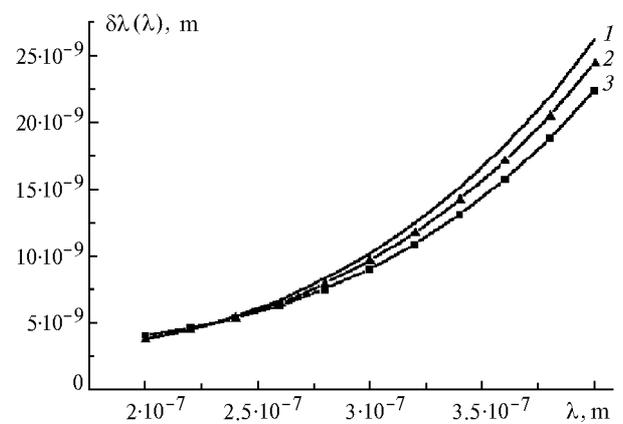
Fig. 4. Spectral resolution at different record parameters of the holographic lens:  $L1 = 35$  (1) and 25 cm (2, 3);  $L2 = 4$  (1, 2) and 3 cm (3).
