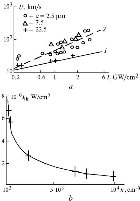
**Fig. 6.** Dependence of the LRAW speed on the radiation intensity (a): LDW (1) and FIW (2); dependence of the threshold intensity of low-threshold optical discharge on the concentration of aerosol particles (b): experimental data (crosses) and calculation (solid line).
