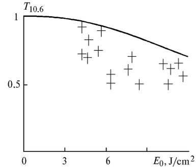
**Fig. 4.** Dependence of  $T_{10.6} = E/E_0$  on the initial energy density  $E_0$ ; calculation by Eq. (13) (solid line);  $b = 1.6 \cdot 10^9 \text{ W} \cdot \mu\text{m}^2 \text{cm}^{-2}$ ,  $k = 2$ ,  $F = 0.5$ ,  $S = 4$ ,  $m = 1/3$ ,  $z = 100 \text{ m}$ .
