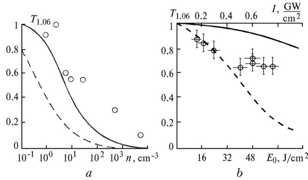
**Fig. 3.** Dependence of  $T_{1.6} = E/E_0$  on the concentration of aerosol particles  $n$  (a) and on  $E_0$  at  $n = \text{const}$  (b). Calculation by Eq. (13) (solid line) and Eq. (12) (dashed line) with the parameters  $b = 2.9 \cdot 10^9 \text{ W} \cdot \mu\text{m}^{1.5} \text{cm}^{-2}$ ,  $k = 1.5$ ,  $S = 4$ ,  $z = 2 \text{ m}$ .
