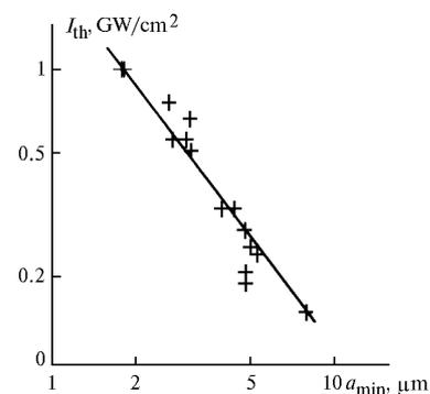
Fig. 2. Dependence of breakdown threshold  $I_{th}$  on the minimum size  $a_{min}$  of aerosol particles taking part in the formation of sparks; calculation by Eq. (1) (solid line).
