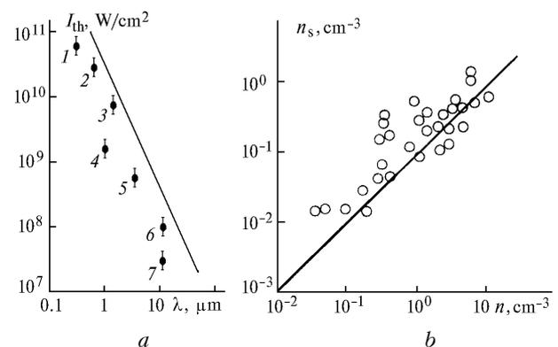
**Fig. 1.** Wavelength dependence of the threshold of a long laser spark occurrence in aerosol media (a): experimental data for air containing aerosol particles (1–7) at  $\lambda = 0.35$  (1), 0.53 (2), 1.06  $\mu\text{m}$  (3) (Ref. 10)  $\lambda = 1.06$  (4), 3.8 (5), 10.6 (6), 10.6  $\mu\text{m}$  (7) (Refs. 8, 9, 11, and 12) and dependence of the concentration of laser sparks  $n_s$  on the concentration of aerosol particles at the pulse energy of 100 J (b).
