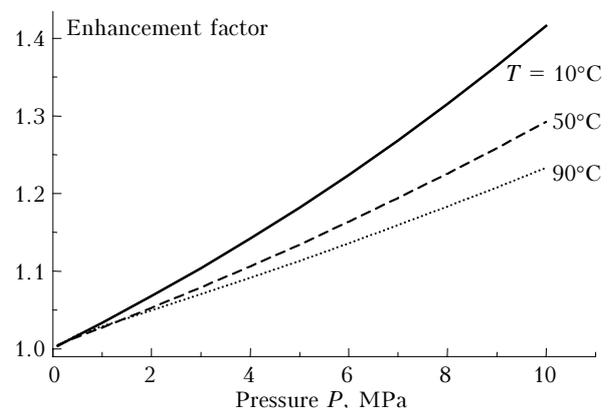
Fig. 1. Pressure dependence of the enhancement factor of moist nitrogen.
