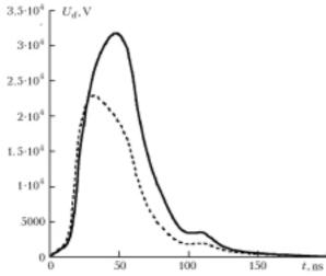
Fig. 5. Time dependence of GDT voltage;  $N_{\rm Cs} = 0\%$  (solid curve) and 1.10<sup>14</sup> cm<sup>-3</sup> (dashed curve).
