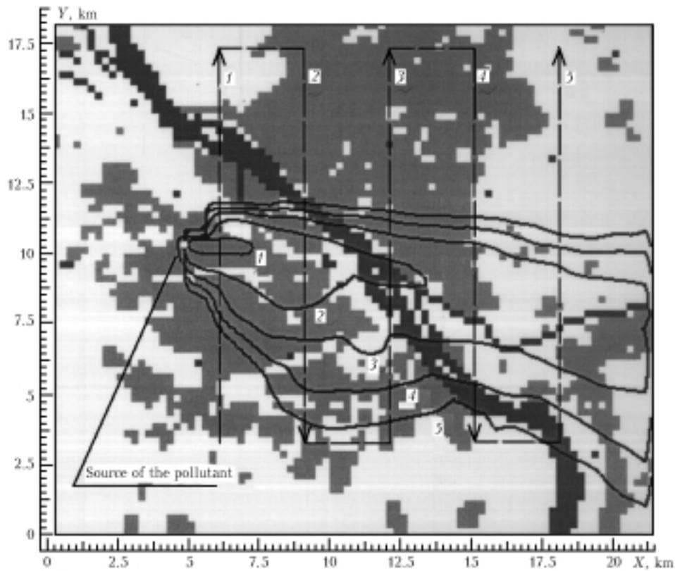
**Fig. 1.** Illustration to the problem formulated. Isolines 1–5 correspond to the pollutant concentrations of  $10^4$ ,  $10^3$ ,  $10^2$ ,  $10^1$ ,  $10^0$  rel. units at the height  $z = 100$  m. The routes of the mobile monitoring network are shown by dashed lines.
