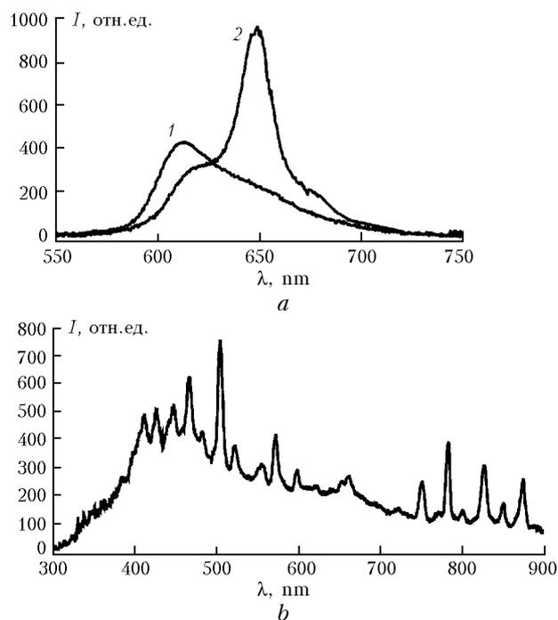
**Fig. 4.** Emission spectra of phenalemine 512 in a PGC drop (*a*) and a spark induced by the focused laser radiation in air (*b*): TPLu (1) and TPL (2).
