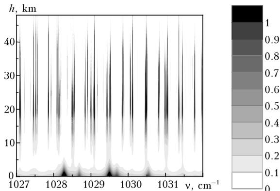
**Fig. 2a.** Height and spectral dependence of the molecular absorption coefficient in the gas mixture of H<sub>2</sub>O, CO<sub>2</sub>, and O<sub>3</sub>, in km<sup>-1</sup>.
