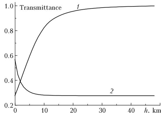
**Fig. 1c.** Calculation of atmospheric transmittance by the line-by-line method. Vertical paths: fixed upper boundary  $h_{up} = 50$  km, variable lower boundary (1); fixed lower boundary  $h_{low} = 0$  km, variable upper boundary (2). Spectral range of 740–760 cm<sup>-1</sup>.
