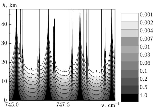
**Fig. 1a.** Height and spectral dependence of the CO<sub>2</sub> molecular absorption coefficient, in km<sup>-1</sup> (fragment of the spectrum).
