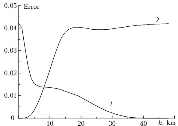
**Fig. 2d.** Error of transmittance calculation by the *k*-distribution method. Designations are the same as in Fig. 1c.
