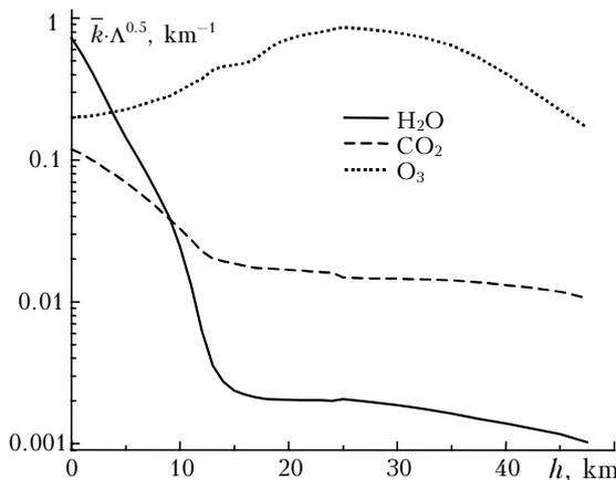
Fig. 4. Height dependence of the mean absorption coefficient multiplied by the lacunarity parameter for different absorbing gases in the spectral range of 1027–1032  $\text{cm}^{-1}$ .
