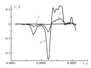
Fig. 3. PA signals generated at absorption of Ti:Sa laser pulses by indoor air.
