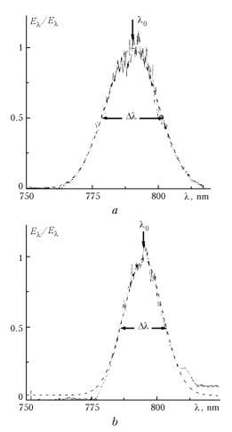
**Fig. 1.** Spectra of Ti:Sa laser pulses with  $\tau_p = 9$  ns (*a*) and 80 fs (*b*): dashed curves are for the results of fitting by the Gauss function;  $\lambda_0 = 790$  nm and  $\Delta \lambda = 23.4$  nm (*a*);  $\lambda_0 = 794.7$  nm,  $\Delta \lambda = 17.7$  nm (*b*).
