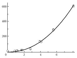
**Fig. 4.** Dependence of the energy of femtosecond Ti:Sa laser pulse absorbed by air on the laser pulse energy  $(a, b, c \text{ are fitting parameters; } R^2$  is the correlation coefficient).
