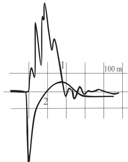
Fig. 1. Current (1) and voltage (2) pulses.
