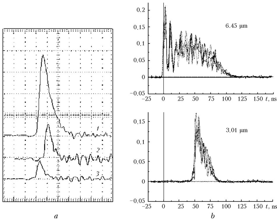
**Fig. 2.** Time dependence of lasing (in rel. units): total pulse (a):  $\lambda \sim 1, 3, 6.45$  ( $1$ ),  $3$  ( $2$ ), and  $1 \mu\text{m}$  ( $3$ ); lasing pulses at the lines  $\lambda = 6.45$  and  $3.01 \mu\text{m}$  (b); the scale graduation of the oscilloscope is  $50 \text{ ns}$ .
