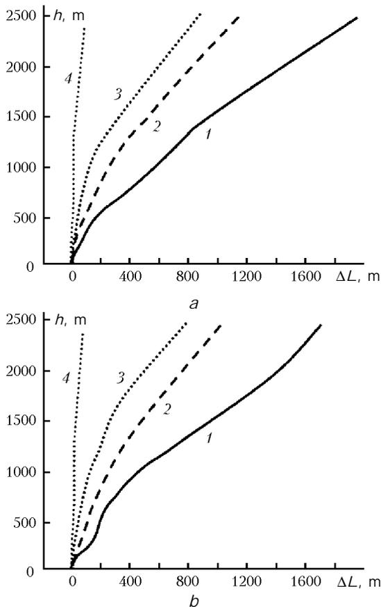
**Fig. 3.** Errors in the visual determination of the range to the viewed object along the earth's surface as estimated from the data of the temperature–wind sensing: nighttime sensing (3 LT) (a), morning sensing (9 LT) (b). Curves 1, 2 are obtained with the allowance for the earth's surface curvature for the viewing angles of  $2^{\circ}40'$  and  $3^{\circ}15'$ ; curves 3, 4 are obtained neglecting the earth's surface curvature for the viewing angles of  $2^{\circ}40'$  and  $3^{\circ}15'$ .
