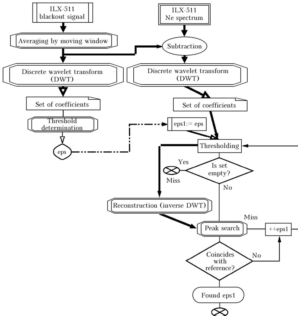
Fig. 2. Algorithm for selection of filtering coefficients.
