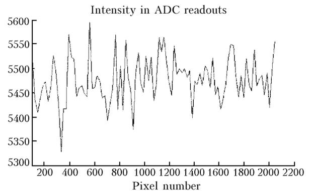
Fig. 4. Result of filtering by the moving window of an extra-weakened signal.
