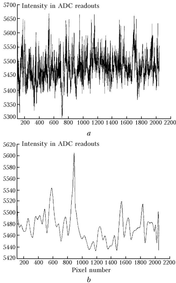
Fig. 3. Initial (a) and filtered (b) weak signals.
