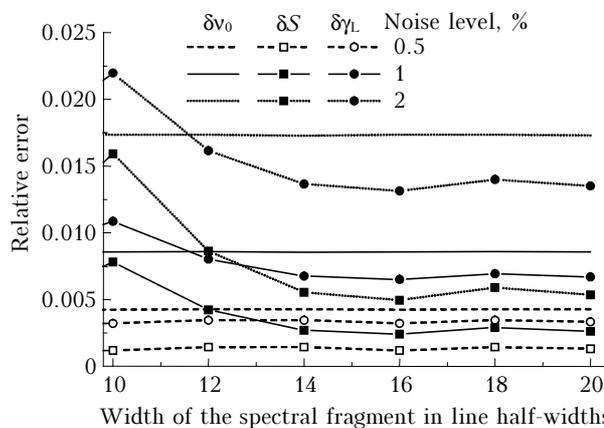
Fig. 4. Errors of retrieval of line parameters vs. width of the spectral fragment involved in the processing.
