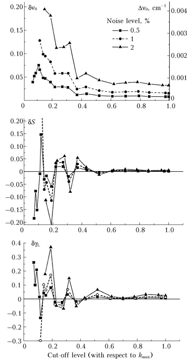
Fig. 2. Errors of retrieval of line parameters vs. cut-off level for the largely Doppler profile ( $\gamma_D = \gamma_L = 0.022 \text{ cm}^{-1}$ ).
