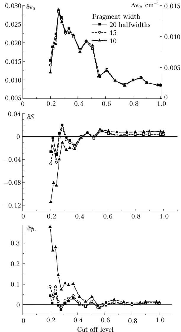
**Fig. 5.** Errors of retrieval of line parameters vs. cut-off level and the spectral fragment width for the Lorentz profile.
