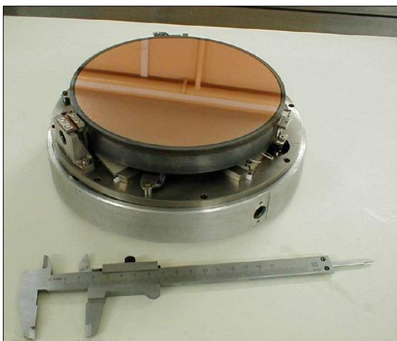
Fig. 8. Bimorph mirror for imitation of wave front distortions.
