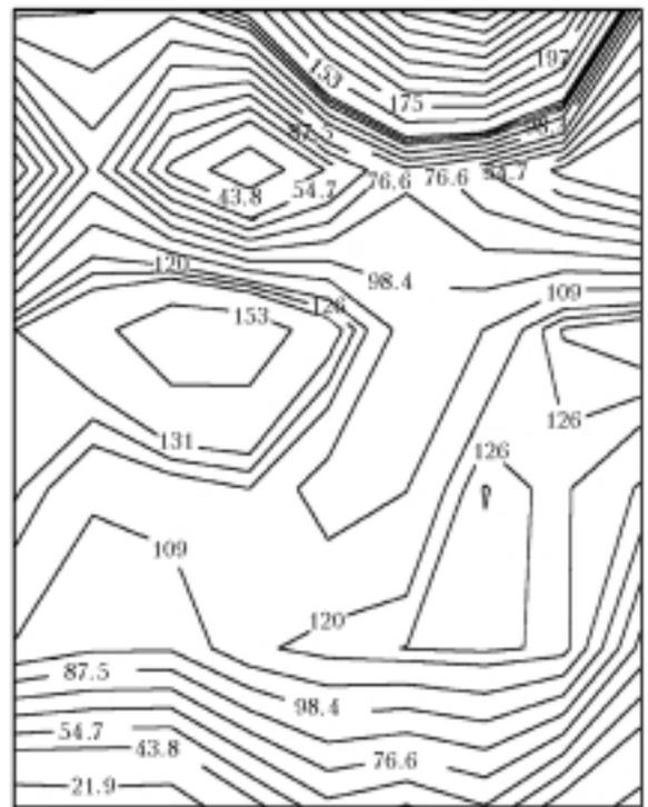
Fig. 6. Distribution of nucleation mode at the height of 400 m, cm<sup>-3</sup> (see coordinates of the plate in Fig. 3).
