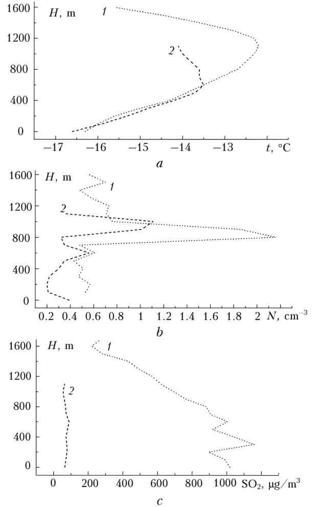
Fig. 2. Vertical distributions over Norilsk on November 10, 2002 of air temperature (a), aerosol number density ( $d \geq 0.4 \mu\text{m}$ ) (b), sulfur anhydride concentration at take off (1) and landing (2) (c).
