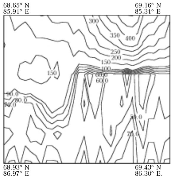
Fig. 3. Distribution of the sulfur anhydride concentration at the height of 400 m on November 10, 2002,  $\mu\text{g}/\text{m}^3$ .
