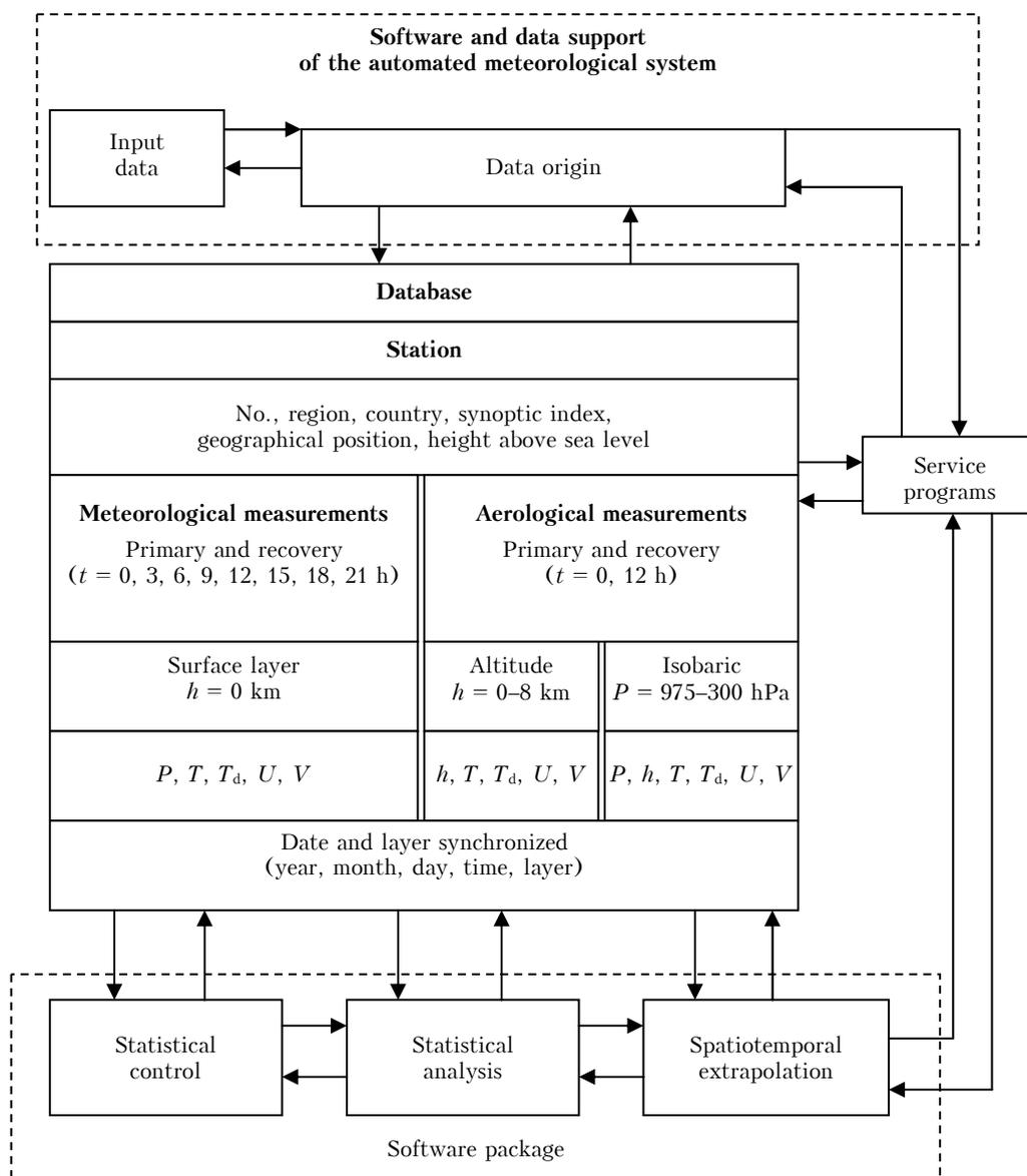
Fig. 1. Block-diagram of meteorological and aerological databank.
