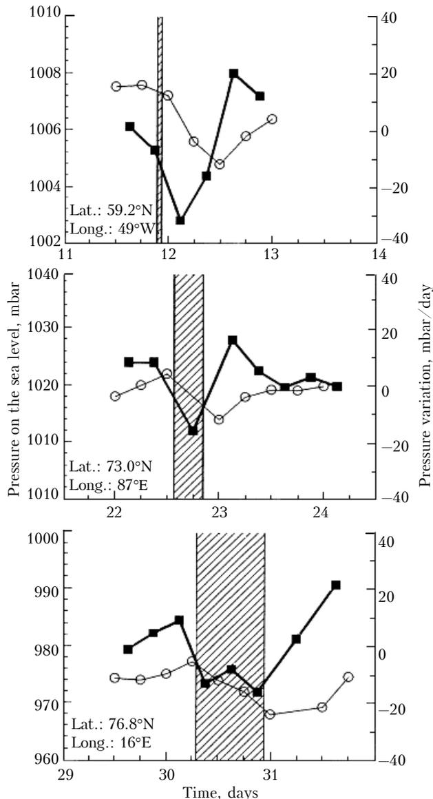
**Fig. 8.** Relation of the atmospheric pressure behavior to the ionospheric disturbances in January 2000.<sup>25</sup> The pressure variations at the sea level (○); the variations of its derivative with respect to time (■). Periods of ionospheric disturbances observed in the X-rays are shown by shadow area.
