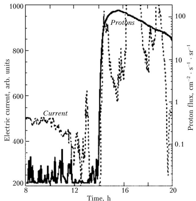
**Fig. 3.** Variations of the ionosphere – Earth electric current density in a polar region in period of increased flux of the solar cosmic rays on April 15, 2001.<sup>16</sup>
