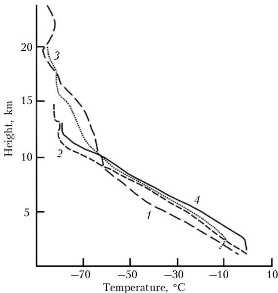
**Fig. 5.** Variations of the temperature vertical profile after the SCR intrusion into the high-latitude region in the period of February 15–18, 1984: before the solar cosmic rays invasion (1); after the SCR invasion (2–4).
