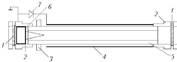
**Fig. 2.** Schematic presentation of the laser chamber: 1 are the mirrors of the laser cavity; 2 are the brass electrodes; 3 is the insulator; 4 is the copper braiding; 5 is the ceramic tube; 6 is the copper ring with the Y-shaped cathode; 7 is the SOS-diode.
