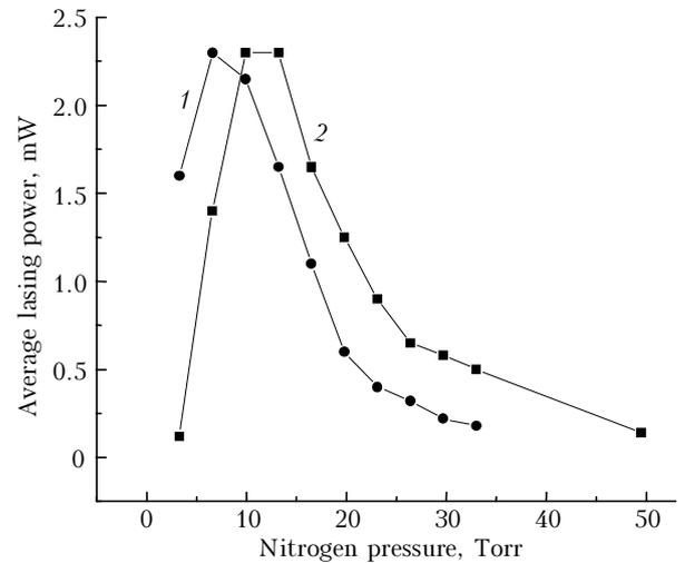
**Fig. 5.** Dependences of the average radiation power of the nitrogen laser pumped by longitudinal discharge on the active medium pressure for two Y-shaped cathodes of various length:  $d$  equal to 23 mm (1); to 100 mm (2). Pulse-periodic mode at the pulse repetition frequency of 10 Hz.
