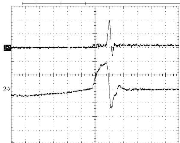
**Fig. 3.** Oscillograms of voltage pulses (1) on the anode of a laser head (vertical scale 65 kV/div) and current (2), running through the SOS-diode and shunt  $R_{sh1}$  (vertical scale 620 A/div) under no-load conditions. The horizontal scale is 50 ns/div.
