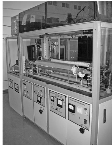
**Fig. 1.** External view of the research SrVL system for resonance ablation of biological tissues and polymers.
