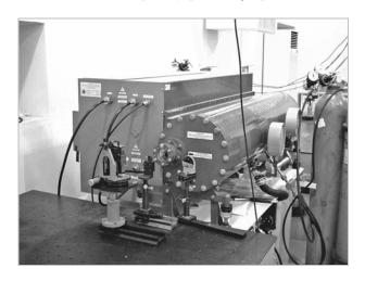
sides near the anode. The energy bulk for the active medium comes from a 550 nF accumulator charged to 18 kV. The cavity consists of mirrors with a dielectric coating, whose reflection coefficients are 100 and 20%. In the mixture Ne : Xe : HCl = = 1520 : 10 : 1 used at a pressure of 2 atm the peak laser generation energy exceeded 1.5 J at a pulse duration of 300 ns and the overall efficiency of 1.35%.
