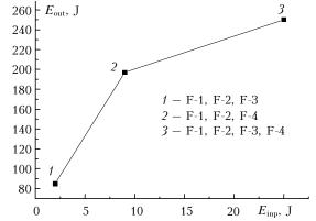
Fig. 3. The output energy of Foton-5 under a double-pass amplification versus the strength of the input signal.
