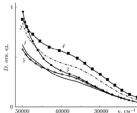
**Fig. 1.** Absorption spectrum of HS in the water-alkaline solution at  $C_{\text{HS}} = 0.0098$  g/l,  $C_{\text{NaOH}} = 0.0019$  m/l: HS from the Merck peat (1), chernozem (2), sod-podzol (3), brown coal (4), and podzol (5).
