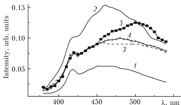
**Fig. 2.** Fluorescence spectrum of HSs in water-alkaline solutions  $C_{\text{HS}} = 0.0098 \text{ g/l}$  and  $C_{\text{NaOH}} = 0.0019 \text{ m/l}$ ;  $\lambda_{\text{pump}} = 365 \text{ nm}$ ; HS from the Merck peat (1), chernozem (2), sod-podzol (3), brown coal (4), and podzol (5).
