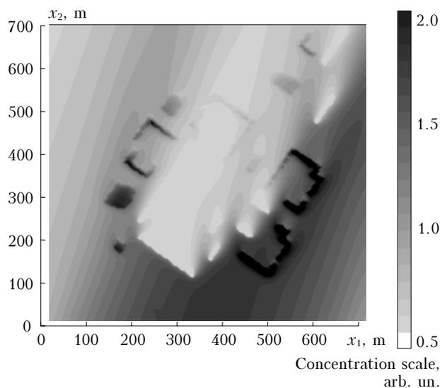
Fig. 3. Calculated normalized concentration field delivered by the external flow.
