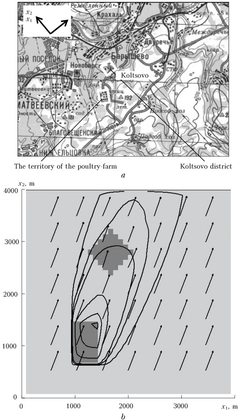
**Fig. 1.** The fragment of the region topographical map (a) and the example of calculation of the fields of wind speed and contaminant concentration cross section at a height of 2 m above the underlying surface (b).
