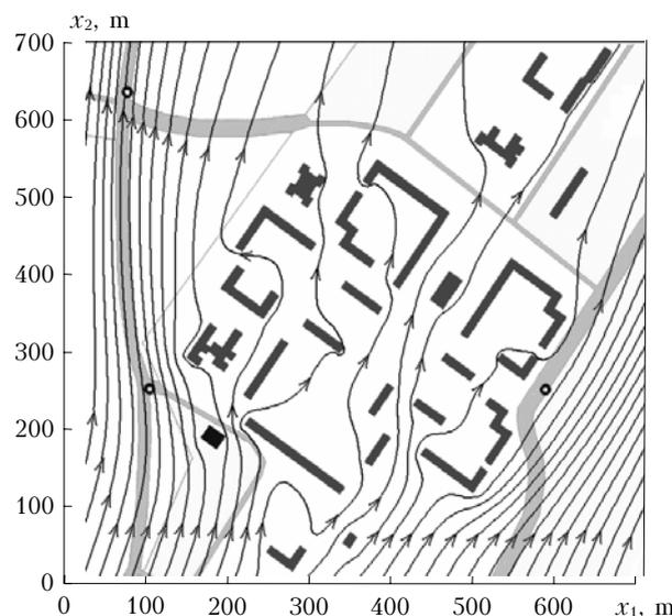
Fig. 2. Isolines of current function in the Koltsovo district in conditions of a strongly stable stratification.
