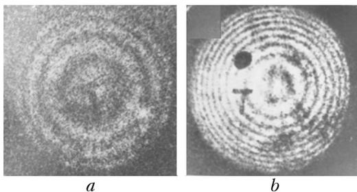
**Fig. 7.** Interference patterns, localized in the plane of the diffuser image formation and characterizing its longitudinal motion: for the distance  $l_2 = 300$  mm (a); for  $l_2 = 180$  mm (b).
