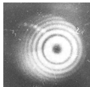
Fig. 9. Interference pattern, localized in the plane of the Fourier hologram and characterizing the cross and longitudinal motions of a flat diffuser.
