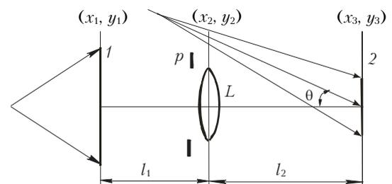
**Fig. 1.** Diagram of the double-exposure recording of the quasi-Fourier hologram: 1 is the matte screen; 2 is the photographic plate;  $L$  is the positive lens;  $p$  is the aperture diaphragm.
