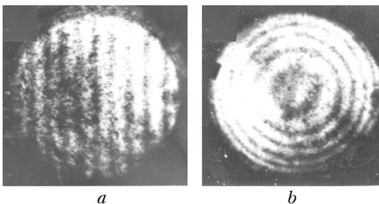
**Fig. 5.** Interference patterns, localized in the hologram plane and characterizing: the cross motion of the diffuser (*a*); the longitudinal motion of the diffuser (*b*).
