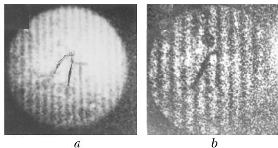
**Fig. 6.** Interference patterns, localized in the plane of the diffuser image formation and characterizing its cross motion: for the illumination of the diffuser with radiation of a diverging spherical wave (*a*); for the case of illumination with a converging spherical wave (*b*).
