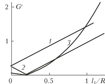
**Fig. 3.** Dependences of the interferometer sensitivity coefficients at the fixed values of  $f = 220$  mm,  $l_1 = 220$  mm,  $l_2 = 180$  mm:  $G_1'$  (1),  $G_2'$  (2),  $G_3'$  (3).
