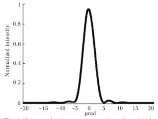
Fig. 4. This graph is a cross section through the (normalized) peak intensity of a far-field beam numerically propagated from a  $3 \times 10^3$  m ground site to  $10^6$  m. The simulation wavelength was 1.0  $\mu$ m and the aperture was 0.25 m. Ten atmospheric phase screens were used. There is minimum corruption when compared to a vacuum-propagated, diffraction-limited beam.
