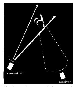
Fig. 1. This figure shows a scenario for a ground–space– ground laser illumination experiment. A laser is fired through a ground telescope (transmitter) at an orbiting satellite. The reflected light is collected by a detector (receiver) on the ground. This received time-series signal is used to compute the pointing errors of the laser transmitter. A typical range to a satellite is  $10^6$  m and the transmitter and receiver separation is 100 m.
