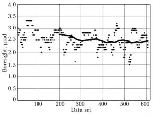
**Fig. 6.** This plot shows the boresight estimate (black dots) for each data set (from 25 measured intensities) for the IRAS data shown in Fig. 3. The 200-point running average (solid line) indicates a large pointing offset of ~2.5  $\mu$ rad. This was determined to be due to the engagement geometry and passive tracking with the transmitter-satellite-sun angle at approximately 90°.
