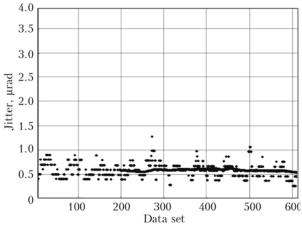
**Fig. 5.** This figure shows the jitter estimate for the IRAS engagement in Fig. 3. Each black dot shows the jitter estimate from a data set. Each data set is from 25 measured intensities. The 200-point running average is indicated by the solid line. The jitter estimate of approximately 0.6  $\mu$ rad indicates very good atmospheric seeing and excellent tracker performance during the satellite pass.
