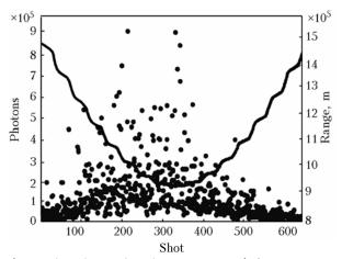
**Fig. 3.** This shows the photons measured from an IRAS engagement (black dots) performed during a recent experiment in New Mexico, USA. The range (R) to the satellite is shown by the solid line and is not smooth since the data was recorded by shot number instead of time. More photons are measured as the satellite comes closer to the observer due to the  $R^4$  effect.
