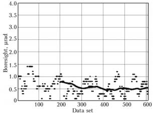
Fig. 7. This plot shows each data set (25 point) boresight estimate (black dots) for the IRAS data shown in Fig. 3, but with a 2  $\mu$ rad solar offset included in the model. The 200-point running average (solid line) indicates a small pointing offset of ~0.5  $\mu$ rad.
