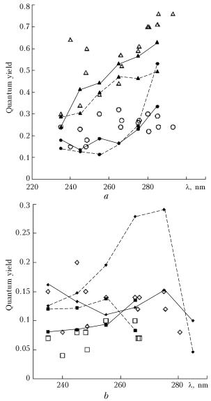
**Fig. 1.** Quantum yields of the  $O_2(a^1\Delta_g, v = 0-3)$  molecules, calculated within the framework of classical and quantummechanical approaches<sup>8</sup>: v = 0 and 1 (a); v = 2, 3 (b). Symbols are the experimental data (see Table 2): triangles (v = 0), circles (v = 1), rhombuses (v = 2), squares (v = 3), curves with the corresponding symbols are the theoretical calculation from Ref. 8 (solid lines represent the classical approach, dashed lines the quantum-mechanical approach).
