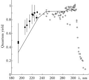
**Fig. 3.** Experimental data on quantum yields of the O(<sup>1</sup>D) atoms: squares together with the values of errors (Ref. 9), circles (Ref. 10); line is the total quantum yield of the  $O_2(a^{1}\Delta_{g}, v)$  molecules, calculated by the approximating formulas.
