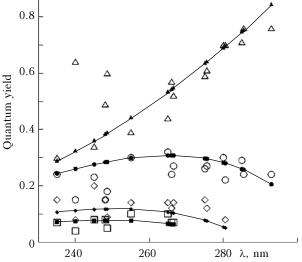
**Fig. 2.** Quantum yields of the  $O_2(a^1\Delta_g, v = 0-3)$  molecules, calculated by the approximating formulas (14). Symbols are the experimental data (see Table 2): triangles (v = 0), circles (v = 1), rhombuses (v = 2), squares (v = 3), curves with corresponding symbol represent the data calculated by formula (14).
