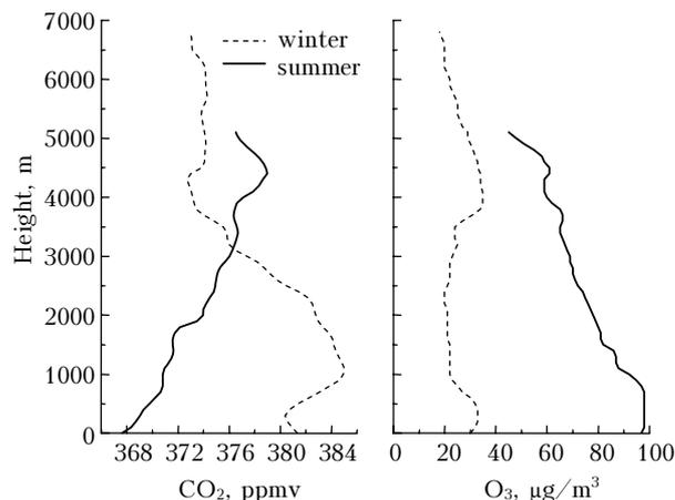
**Fig. 4.** Vertical distribution of carbon dioxide and ozone in November 2002 and August 2004.
