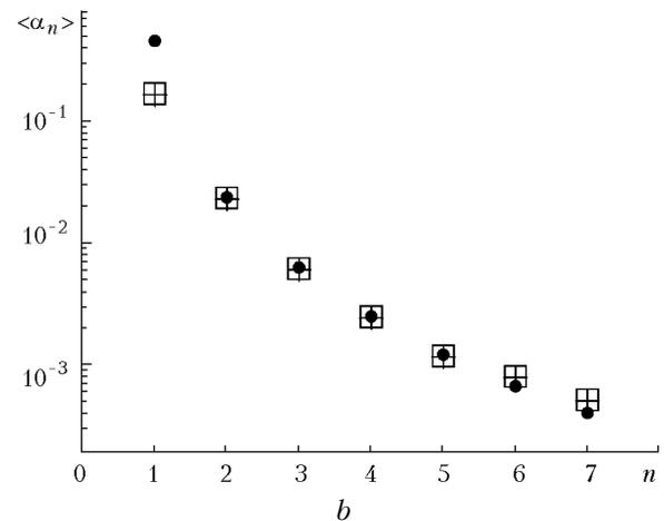
Fig. 3. Normalized coefficients  $\langle \alpha_n \rangle$  of screens expansion over Zernike polynomials: normalizing to  $\sigma_1^2$  sum (□); normalizing to  $\sigma_2^2$  sum (+); theoretical values (●).
