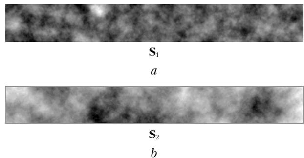
Fig. 1. Phase screens of  $128 \times 1024$  pixels size generated using pulsed response function  $\mathbf{H}$  of different widths:  $\mathbf{S}_1$  screen was obtained with  $\mathbf{H}$  of the width equal to 128 (a) and screen  $\mathbf{S}_2$  using  $\mathbf{H}$  of the width equal to 512 (b).
