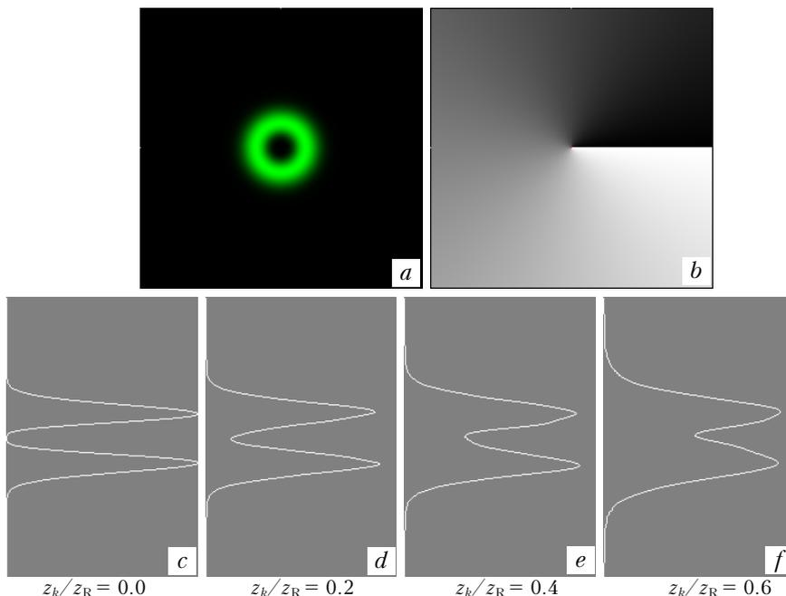
**Fig. 2.** Intensity (a) and the phase (b) of the initial collimated vortex beam with  $l = 1$ ; profiles of the beam intensity calculated for some propagation distances  $z_k/z_R = 0.0; 0.2; 0.4; 0.6$  (c–f) using the values of the dimensionless parameter  $C_T^2 = 0.1$ .
