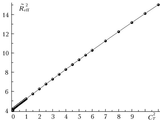
**Fig. 3.** Dependences of  $\tilde{R}_{\text{eff}}^2(C_T^2)$  for vortex beams at  $z_k/z_R = 0.2$ .
