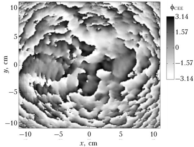
**Fig. 3.** Distribution of the phase of a Gaussian beam field unwrapped using the Fried's complex exponential phase estimator.<sup>9</sup>
