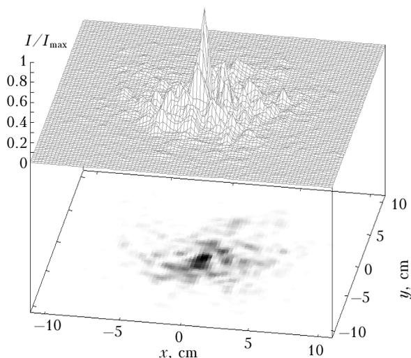
Fig. 7. Intensity distribution of a Gaussian beam after backward propagation if conjugating only the phase unwrapped using the LSM.
