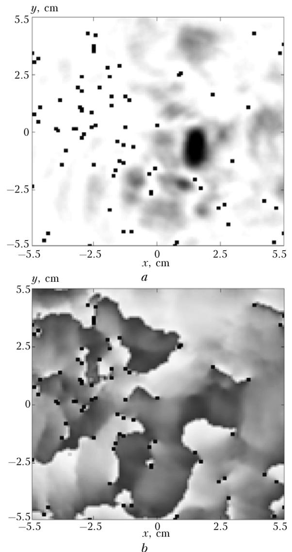
**Fig. 4.** Intensity (a) and phase (b) distributions in the central part of the beam cross section with the marked branch points of the phase.
