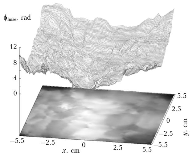
**Fig. 5.** LSM-unwrapped phase distribution.
