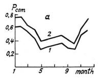
FIG. 3. Annual behaviour of communication probability in Tompo. 1-5 dB attenuation, 2-50 dB attenuation.
