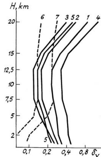
FIG. 5. The relative error  $\delta_v$  versus the altitude  $H$  for a space-lidar. For curves 6 and 7  $v(H) = 30 m/sec$ ; for the other curves see the caption to Fig. 4.
