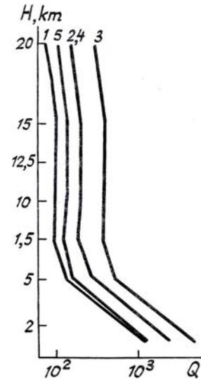
FIG. 4. Profiles of the SNR  $Q$  for a space-based lidar.  $E = 0.5 J$  (1, 7), 1 (2, 4, 5, 6), and 2 (3); for curves 5 and 6  $\varphi^* = 45^\circ$  and for the other curves  $\varphi^* = 30^\circ$ ; for curve 4  $\xi = 200$  and for the other curves  $\xi = 100$ ;  $\Delta R = 1500 m$ .
