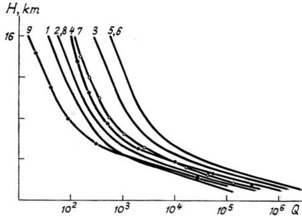
FIG. 2. Profiles of SNR  $Q$  for ground-based lidar.  $E = 0.065 J$  (1),  $0.1$  (2, 8, 9),  $0.5$  (3, 4, 7), and  $1$  (5, 6); for curves 4 and 9  $C_{n0}^2 = 10^{-12} m^{-2/3}$  and for the other curves  $10^{-14} m^{-2/3}$ ; for curve 8  $\xi = 200$  and for the other curves  $\xi = 100$ ; for curve 7  $\Delta R = 300 m$  and for the other curves  $750 m$ .
