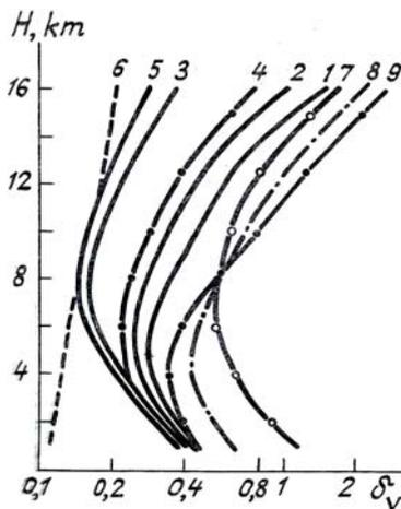
FIG. 3. The relative error  $\delta_v$  versus the altitude  $H$  for a ground-based lidar. For curve 6  $v(H) = 30 m/sec$ ; for the other curves see caption to Fig. 2.
