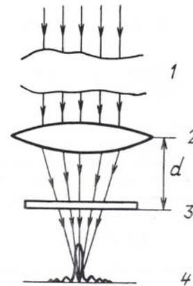
FIG. 1. Schematic of Image Correction: 1) distorting medium; 2) lens; 3) phase corrector; 4) image plane.
