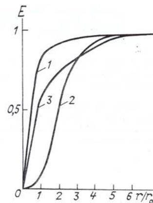
FIG. 3. Energy distribution over the blur circle: 1) no distortions; 2) phase fluctuations with  $D_s(\emptyset) = 5.26 \text{ rad}^2$ ; 3) phase correction by adaptive mirror;  $r_0$  is the Airy radius.
