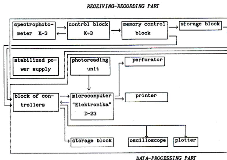
FIG. 1. A structural diagram of the spectral measuring system.
