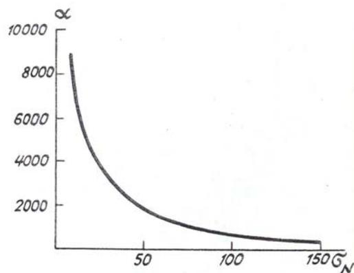
FIG. 3b. Dependence of the optimal parameter of the Gaussian filter  $\alpha$  on the standard deviation of the noise  $\sigma_n$ .
