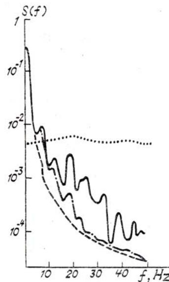
FIG. 2. Spectral densities of the signal model (at a different halfwidth of the instrument function) and noise of the spectral measuring system: the solid curve is the extraterrestrial solar radiation  $I_0$ ; the dashed curve is  $I_0 * A (A/2 = 7 \text{ nm})$ ; the dash-dotted line is  $I_0 * A (A/2 = 2.5 \text{ nm})$ ; and the dotted line is the noise.
