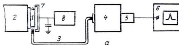
FIG. 1a. Block diagram of the experimental setup: 1) active element; 2) electron beam; 3) optical waveguide; 4) spectral device; 5) PMT; 6) oscilloscope; 7) Faraday cylinder; 8) voltmeter.
