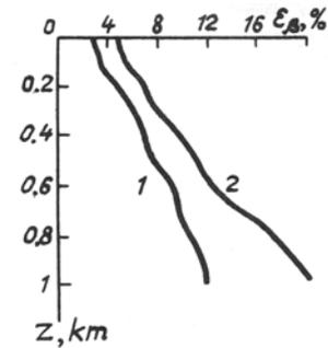
FIG. 3. The error, averaged over the layer, in the reconstruction of  $\beta(x, z)$  versus the penetration depth in the scattering medium:  $\varepsilon = 5\%$  (1) and  $\varepsilon = 10\%$  (2).
