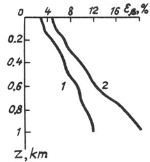
FIG. 3. The error, averaged over the layer, in the reconstruction of  $\beta(x, z)$  versus the penetration depth in the scattering medium:  $\epsilon = 5\%$  (1) and  $\epsilon = 10\%$  (2).
