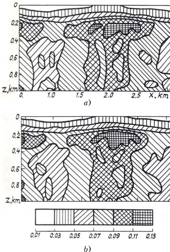
FIG. 2. The reconstruction of the two-dimensional spatial distribution of the backscattering coefficient  $\beta(x, z)$  in a numerical experiment: a) model distribution  $\beta_0(x, z)$ ; b) result of the solution of the inverse problem with a 10% error in the lidar signals.
