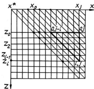
FIG. 1. A discrete scheme for two-beam tomographic sounding of the atmosphere.
