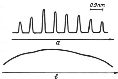
FIG. 2. Lasing spectra with Brewster (a) and normal (b) orientation of faces of the active element.
