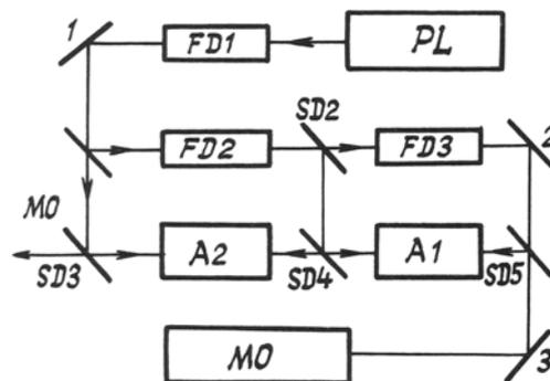
FIG. 4. Block diagram of a multifrequency laser: PL — pump laser; FD1–FD3 — frequency doublers; 1, 2, 3 — mirrors; SD1–SD5 — spectrum dividers; A1, A2 —  $\text{Al}_2\text{O}_3:\text{Ti}^{3+}$ -based amplifiers; MO —  $\text{Al}_2\text{O}_3:\text{Ti}^{3+}$ -based master oscillator.
