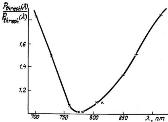
FIG. 1. The lasing threshold versus the wavelength of a  $\text{Al}_2\text{O}_3:\text{Ti}^{3+}$  gased laser.
