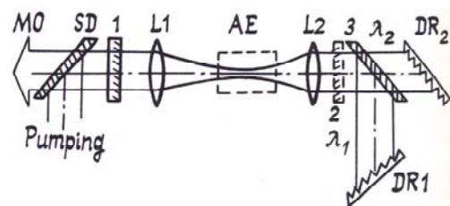
FIG. 3. The optical layout of multifrequency laser based on  $\text{Al}_2\text{O}_3:\text{Ti}^{3+}$ : SD - spectrum divider; 1, 2 - resonator mirrors; AE - active elements; L1, L2 - lenses; 3 - beam splitter; DP1, DP2 - autocollimation gratings; AE - active element.
