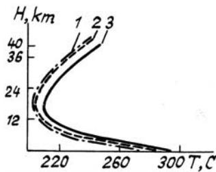
Fig. 2. The vertical temperature profiles obtained in the framework radiative-convective model (RCM) as compared with the standard profile: 1 – RCM, a simplified algorithm; 2 – RCM,  $\Delta$ -Eddington technique; 3 – the standard atmosphere, USA, 1962, 45° of the north latitude, July.
